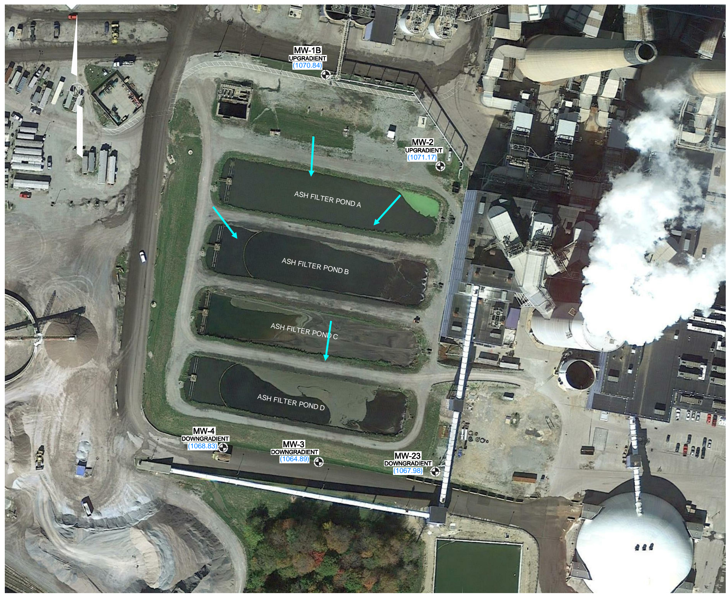
FIGURE 2 CCR COMPLIANCE GROUNDWATER MONITORING WELL LOCATION MAP ASH FILTER PONDS CONEMAUGH GENERATING STATION INDIANA COUNTY, PENNSYLVANIA
